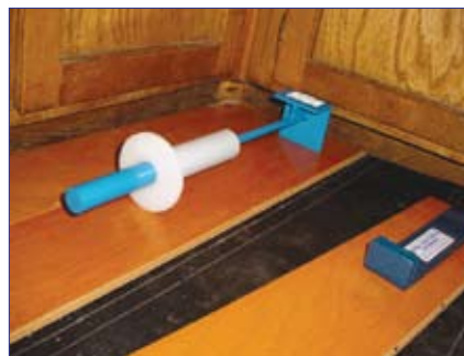
Showing how the tool doesn't fit under the toe kick without the extension.
